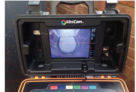
All valves must have CCTV inspection post fitment to ensure correct alignment in situ
